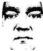
Fig. 2. The original image in Fig. 1 is binarized under the contrast criterion. The percentage of the bright pixels is 80%.
